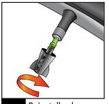
Reinstall valve core.
