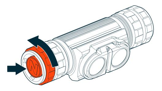
**OPERATION** Press the power button once to turn unit on or off.
