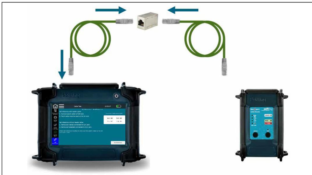
Figure 39 - Test setup for setting the reference - Cu
