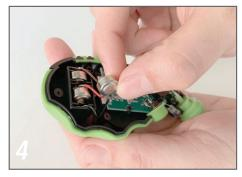
Remove old batteries from gauge being careful not to break small battery contact wires.
