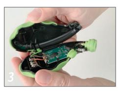
Pull both gauge halves apart completely to expose batteries.
