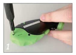
Remove 4 screws from back of gauge body.
