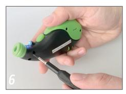
Rejoin gauge halves taking care not to pinch any wires. Reinsert and tighten 4 gauge body screws.
