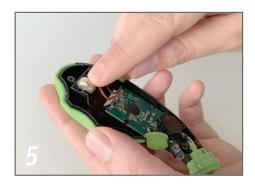
Insert 3 new L1154F batteries into gauge with positive side facing the top of the gauge.
