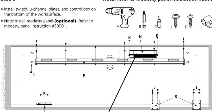
Table will **NOT** operate unless the control box is screwed tight into
