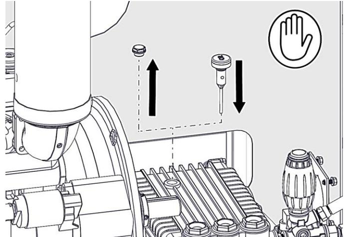
8. Check the oil level in the pump using the dipstick or the sight glass on the back / side of the pump. Make sure the level is between min/max level notches on the dipstick, or is level with the indicator on the sight glass. If oil reservoir needs replenishing only use oil of a type as listed in the data sheet in this instruction manual.
