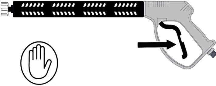
3. Check that the pressure indicated on the pressure gauge matches the value on the data plate in the technical data. Also check that when the trigger is released the pressure shown on the gauge returns to zero.
