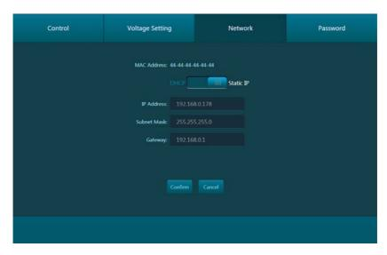
In this interface, dynamic or static IP mode can be selected. Under static IP mode, IP address, subnet mask, and the gateway can be set. Make sure the IP addresses are unique to avoid any IP conflicts.
