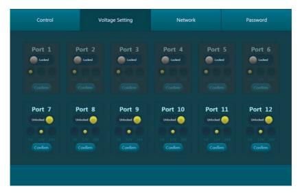
In this interface, you can select **5V**, **12V**, or **24V** for each output channel. Locking the individual ports will prevent changing of the voltages from the rear panel or the web GUI until they are unlocked.
