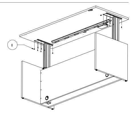
• Install divider cover and worksurface grommet insert.
