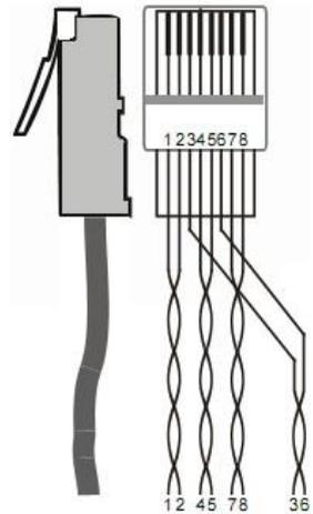
**Note:** For best operation, the twisted pair cable should be shielded and the cable connectors should be metallic. The shielded layer of cable MUST be connected to the connector's metal shell.
