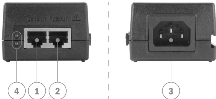
1. Using existing Ethernet cable, connect a LAN port on your non-PoE switch to the Data In port on the injector.
