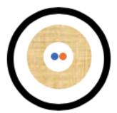
*M3I-2M-P-BK* fiber optic cable is constructed with two internal tight buffers, internal aramid yarn, and one outer plenum-rated PVC jacket in distribution format. The cable features a water-resistant jacket and is designed for indoor and outdoor applications.
