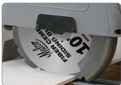
A lower number of teeth and deeper gullets produce cleaner, more precise cuts resulting in an accurately matched trim edge and tighter seams. Perfectly tensioned, hardened tool-steel blade assures a flat true run.
