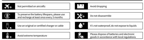
The HALO Power Station 1200 meets all legal requirements for the transportation of dangerous goods. The capacity of the lithium battery pack exceeds 100Wh. According to international standards, if the power station is transported by air, it must be transported in accordance with IATA standard packaging. The instructions and labeling requirements of the International Air Transport Association and related declarations must be completed.
