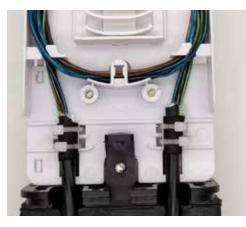
5. Secure the cable to the splice tray with the zip ties wrapping around the foam insulation.
