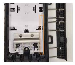
A fiber feed rod (orange rectangle) is attached to the splice tray.
