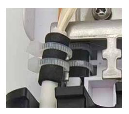
2. Apply Foam insulation to drop. Then secure drop to metal bracket with two of the provided zip ties. \*\*\*Failure to apply foam will allow drop cable to slide.\*\*\*
