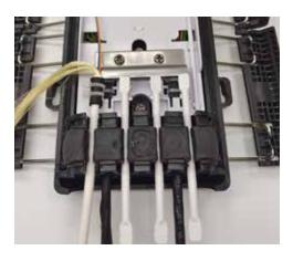
3. Install the included port plugs for any open drop cable ports.
