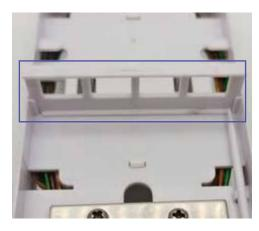
1. Flip the splice tray over and remove the adapter bracket (blue rectangle) if it is installed.
