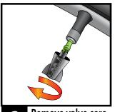
Remove valve core with included tool.
