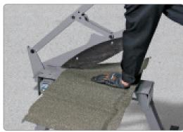
A hardened steel blade and die offer reversible cutting edges for twice the cutting life, prior to sharpening. With the blade lock-pin in place, this portable cutter is safe to transport and sets up virtually anywhere on the job site. Designed with two different length leg tubes to provide the user with two height options. A large table surface allows sure handed control and prevents damage to the work-piece. The table's "feed-thru" design also allows long angle cuts for roof hips and valleys.
