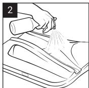
Rinse thoroughly with clean water to remove all residue and dry with a clean lint free cloth. (Scuffing paste residue must be removed completely before top coating. Failure to do so may result in adhesion failure)
