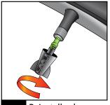
Reinstall valve core.
