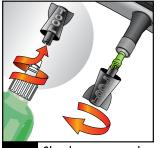
2 Slowly remove valve core with tool in cap.
