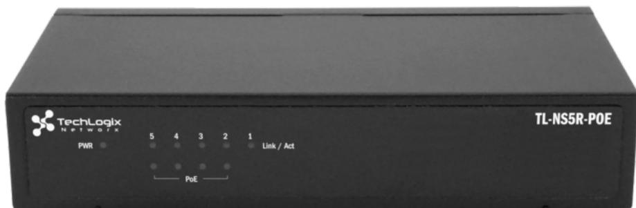
The TL-NS5R-POE is designed to take power from a PoE switch or power injector and pass both data and electrical power to a number of PoE-compatible devices via standard twisted pair cables. Equipped with five Gigabit Ethernet ports, this switch can power up to four wireless LAN access points and bridges, VoIP phones or IP video cameras, draw its own power from the PoE switch it is connected to, and deliver network speeds of up to 1G.
