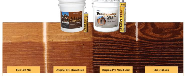
Top half has 1 coat. Bottom half has 2 coats. Left side was sanded smooth. Right side was blasted.
