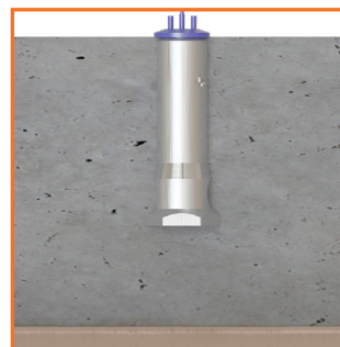
3. "Puddled" into wet concrete
