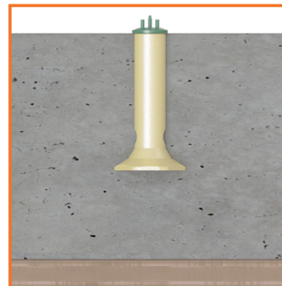
3. "Puddled" into wet concrete
