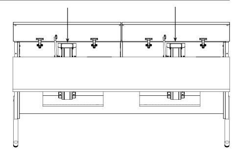
Slide the monitor and motor bracket assembly onto the Column Assembly.
