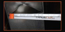
Tip: To apply tape to inside creases, fold your tape in half over the length of the Tight Taper® bar. Align it in the crease and use the orange handle to smooth and secure the tape.
