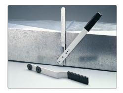
Use the Duct Stretcher to hold duct in place with one hand while slipping drive cleat in place with other hand. The low profile, straight body is designed to go anywhere, even in the tightest quarters. Additional spacing holes allow wheels to be adjusted to span greater distances. Rugged anodized aluminum body features large vinyl cushion grip and handy hang-up hole.
