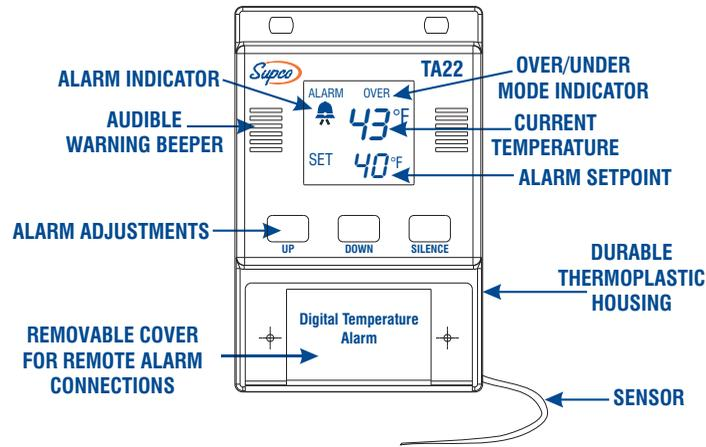
The TA22 Temperature Alarm is a single point or threshold type of temperature alarm. This type of temperature alarm monitors the temperature at the sensor probe tip and when this temperature passes above (or below) the set point, the unit will execute a preset operation.
