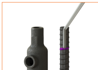
2.b: Dispense half of recommended quantity of epoxy (refer table above) onto the marked end of ReidBar.
