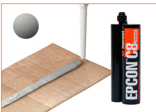
2.a: Dispense initial mix of epoxy from nozzle until a consistent grey coloured mix appears. Discard safely
