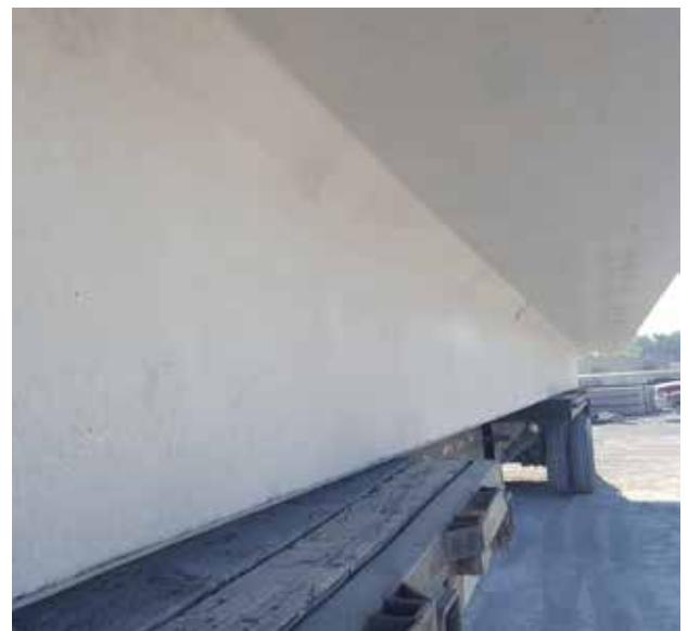
Release Agent #10 used with optimum spray application
