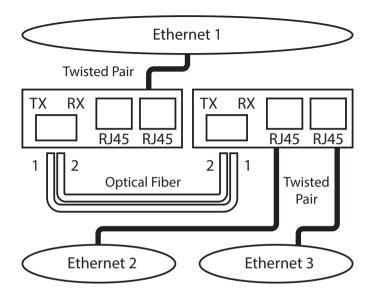
As shown above, two fiber optic cables need to be connected between two ideally identical media converters. Make a connection from Media Converter 1 TX to Media Converter 2 RX, and from Media Converter 1 RX to Media Converter 2 TX.
