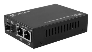
The TL-MC-1S2R features one SFP port (SFP module sold separately) and two RJ45 twisted pair port2, effectively adapting twisted pair-based devices to fiber for longer transmission distances. The TL-MC-1S2R supports multimode fiber when paired with a multimode SFP module and single mode fiber when paired with a single mode SFP module.
