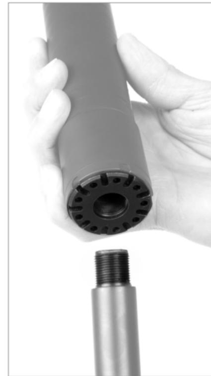
Hold the Harvester Evo body with a firm grip and thread on by hand to avoid cross-threading. Use the three pegs of the Bravo Multitool to tighten the mount to the Harvester Evo body to approximately 20-30 ft-lbs. To remove, perform steps in reverse order.
