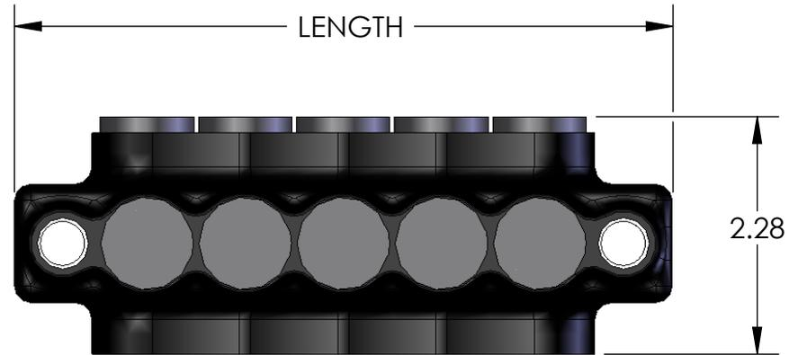
INSULATED MOUNTING PORT ON EACH END FOR A 5/16 BOLT
