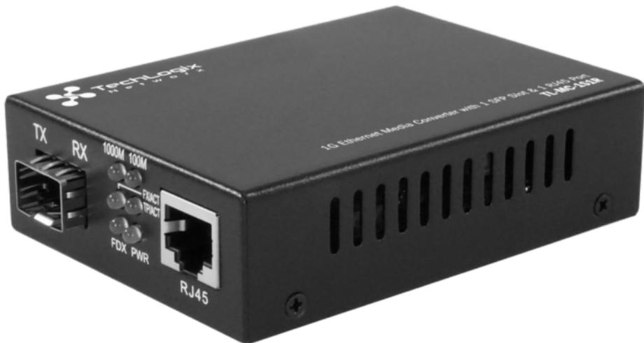
The TL-MC-1S1R features one SFP port (SFP module sold separately) and one RJ45 twisted pair port, effectively adapting twisted pair-based devices to fiber for longer transmission distances. The TL-MC-1S1R supports multimode fiber when paired with a multimode SFP module and single mode fiber when paired with a single mode SFP module.
