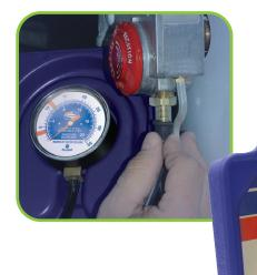
A new Uniweld design feature allows you to easily zero reset the gauge needle by simply twisting and removing the dial lens to access the zero adjusting screw.
