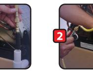
2. Allow Nitrogen (at max. 140 PSIG) to flow through, blasting the sludge free.
