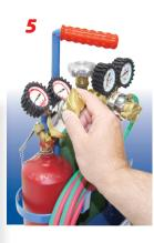
[STEP 5] To shut down the torch for storage or transportation, close the cylinder valves. Release the oxygen pressure by opening the oxygen torch valve [vent safely]. Close the torch valve and repeat this same process for the fuel gas [vent safely]. Close all valves tightly and secure the equipment. *Now the shutdown is complete*!
