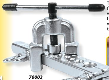
The 70003 Heavy Duty Flaring Tool has a hardened steel flaring cone with a chrome finish for more uniform flares without galling. Special shaped wing nuts allow the long handle of the self-centering yoke to be used as a lever when tightening. The hardened steel flaring bar grips tubing without scoring.
