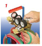
moving. Then, open the valve sufficiently to provide adequate flow. The fuel gas [acetylene] cylinder valve should be opened a maximum of  $\frac{3}{4}$  turn and a wrench should remain in position on the stem of the valve while the cylinder is in use so that the valve can be quickly turned off in case of an emergency.
