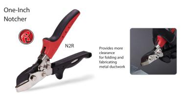
The N2R Notcher punches a big 1 in. (25.4 mm) deep "V" notch in common 24 to 30 ga. (0.71-0.41 mm) galvanized sheet metal quickly and easily.
