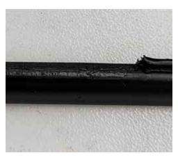
2. Deburr the rough edges of the outer jacket so there will be a tight seal.
