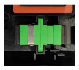
Fiber optic couplers will fit in the center of the enclosure base.
