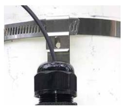
2. Run the clamp band inside the hooks of the mounting brackets. The top to bottom distance is 11 1/2 in.
