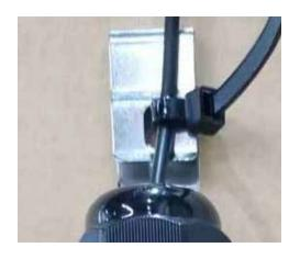
Use a large zip tie to attach the cable to the hook of the mounting bracket as a strain relief. Don't forget to cut off the excess zip tie.
