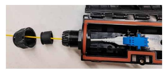
3. Install the cable and connect it to the coupler or keystone jack.
