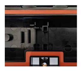
Removing the splice tray reveals some support structures for keystone jacks and fiber optic couplers.
