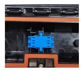
1. Install the appropriate coupler into the enclosure.
