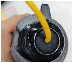
4. Repeat for the other end and thread the sealing nut onto the enclosure hand-tight.
