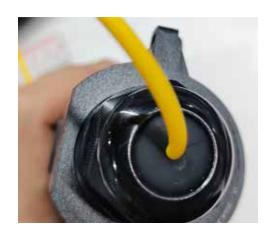
Feed the cable into the enclosure opening and thread the sealing nut onto the enclosure hand-tight. Make sure there are no aramid fibers sticking through the rubber grommet.
