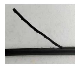
1. Remove 0.5 to 1 m (~1.5 to 3 ft) of the copper trace wire from the cable.
