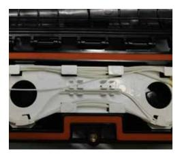
7. Install the fusion splicing tube into the splice tray and wrap the excess fiber in the tray before fusing the ends of the fiber together.
