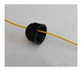
1. Remove the sealing nut from the enclosure and feed it onto the cable.
