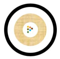
*M3I-6M-R-BK* fiber optic cable is constructed with six internal tight buffers, internal aramid yarn, and one outer riser-rated PVC jacket in distribution format. The cable is designed for indoor applications and features Corning ClearCurve® fiber.
