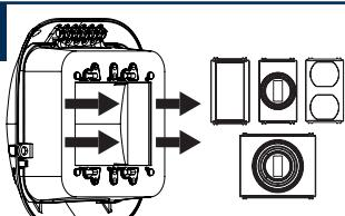
Snap in adapters to accommodate electrical device(s).
