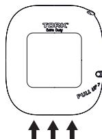
Remove cord knockout(s) with pliers to accommodate cord configuration.
