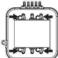
Back out (do not remove) receptacle screws or use screws provided to align base key holes and secure to junction box.
