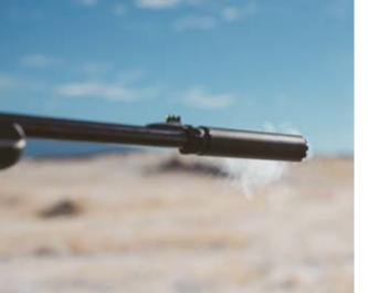
The Spectre 22 mounts on conventional 1/2 X 28 (Class 3A) threads .400" in length.
