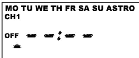
Press **DAY** to show the Sunrise time for today. All days are filled in on the screen. No changes can be made to the day selection. This way the timer always turns off the load at sunrise for energy savings. Even if you created a fixed time off in the SCH section, it a good idea to add the Sunrise OFF.
