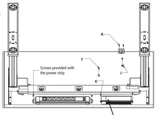
Table will **NOT** operate unless the control box is screwed tight into the table without any play.
