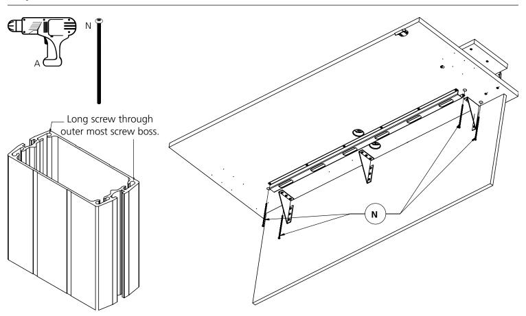
Do not tighten screws until all are installed. Once all screws are installed, tighten four cross support screws and four long screws.
