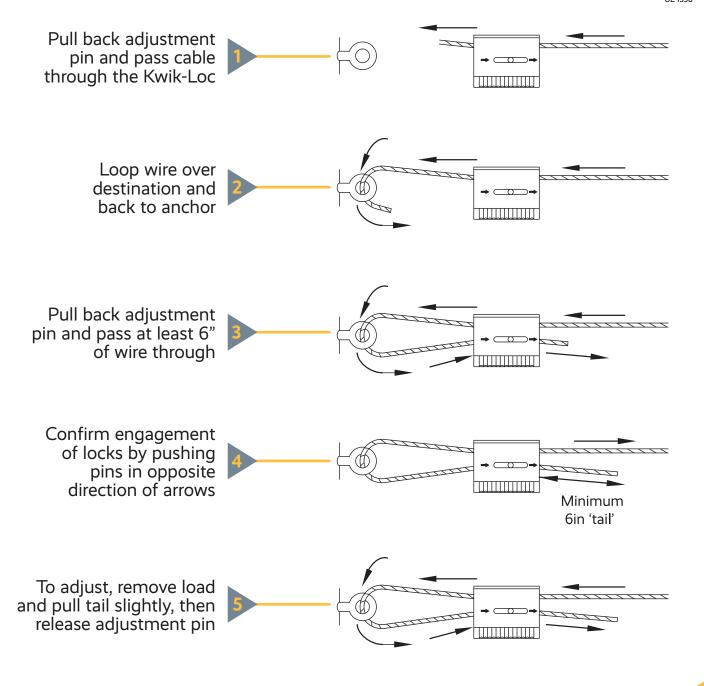
All Duro Dyne Dyna-Tite cable locks have been tested to FIVE times their allowable working load by independent testing laboratories
