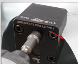
Begin crimping at angle after crease
