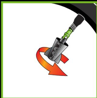
**6** Reinstall valve core.
