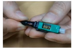
Insert the fiber into the connector body until the strand meets resistance and bows slightly
