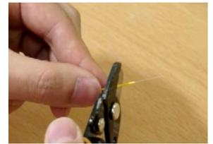
Strip the buffer to the 250µm mark using the middle hole, then the small hole on the stripper in short increments
