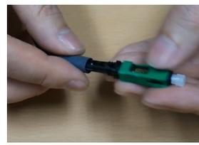
Slide the adapter tube into the connector, then screw the boot onto the connector body and trim any exposed Kevlar yarn
