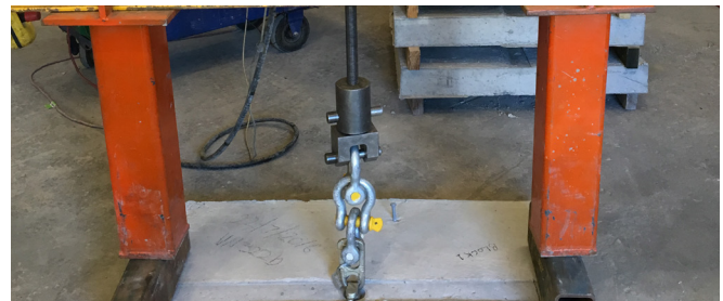
Figure 4: 1FA045 Foot Anchor tested in tension.
