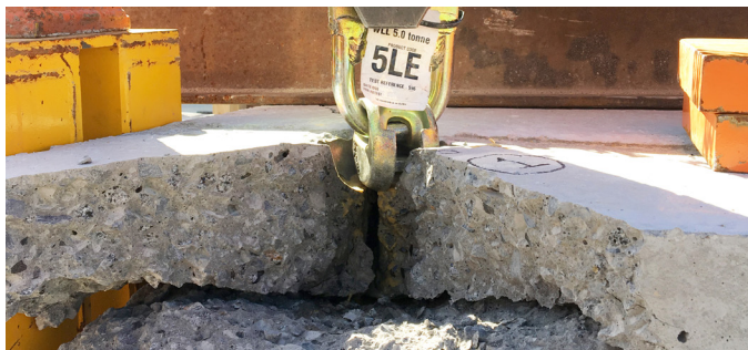
Figure 3: 5FA120 Foot Anchor tested close to an edge.
