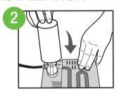
Rotate cartridge into down position.
