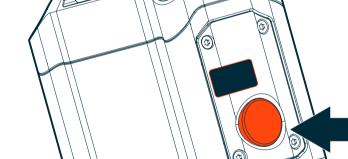
Press power button to turn the unit ON.
