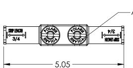
REMOVALBE CAPS FOR ACCESS TO 3/16 INTERNAL HEX PRESSURE SCREWS
