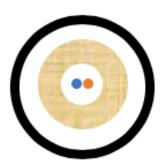
M3I-2M-R-BK fiber optic cable is constructed with two internal tight buffers, internal aramid yarn, and one outer riser-rated PVC jacket in distribution format. The cable is designed for indoor applications and features Corning ClearCurve® fiber.
