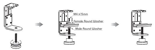
Assemble C Clamp with Mount by driving 3 Screws M5x15mm, flap head, Hex Socket Screws.
